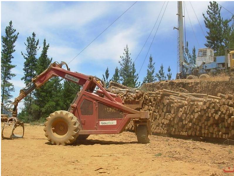
Figure 3.5 Use of “three-wheels” (ergo logger) in medium-sized forest operations.
